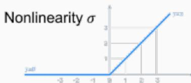
$$n_i = \sigma \left( \sum_{j=1}^m w(x_j, n_i) \cdot x_j \right) = \sigma(\underline{w}_i, \underline{x})$$
